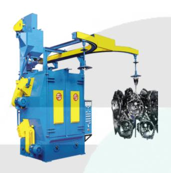
In the competitive world of today's industry, economical surface finishing is important. The ABSS range of Spinner Hanger Blast Machines are designed to handle the cleaning and surface preparation of typically awkward components that cannot be adapted to a Table or Tumble Blast Machines. Parts are loaded onto a hanger and rotated during the blast cycle for multiple angle cleaning.
