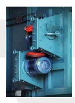
At the heart of the machine there is the dynamically balanced ABSS Blast Turbine that generate the blasting curtain.
