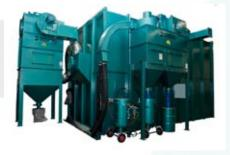
CALL NOW 1300 727 240 The Abrasive Reclaimer is a fully welded steel fabrication which is free standing on its own support structure. This unit performs three basic fuctions:
