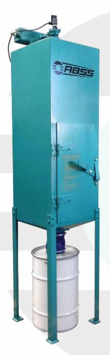
The ABSS Dustech Single Cartridge Dust Collector is a 500CFM free standing unit perfectly sized to suit most standard Abrasive Blast Cabinets in the ABSS range as well as small collection requirements. Also suitable for some non-ABSS Blast Cabinets.
